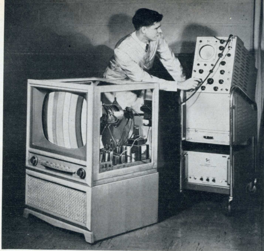
The old Apple tube, developed by Philco around 1956. Somewhat similar principles have been used in later inventions, including the recently announced Goodman tube.
