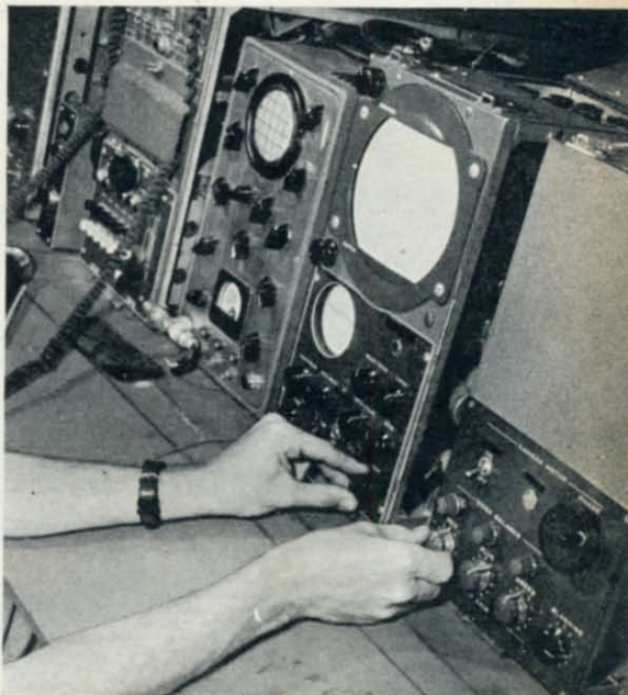
THE CONTROLS An extra panel (extreme right in photo above) adjusts the color-wheel motor and color balance in each camera. The technician's hand is on the knob that sets the amount of red in the picture. Adjacent knobs control blue, green.
