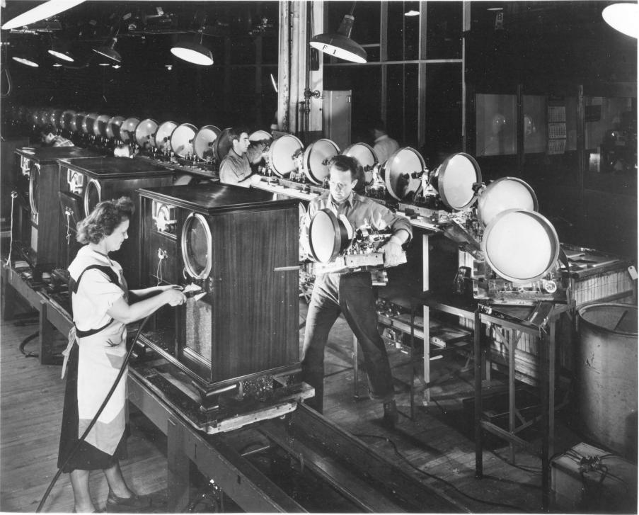
The marriage of TV picture tubes, fine wood cabinetry and complex electronic chassis took place in 1950 at this Chicago manufacturing facility of Zenith Radio Corporation. These sets, featuring TV, FM/AM radio and phonograph, were among the first three-way combination black-and-white sets for home use by Zenith.
