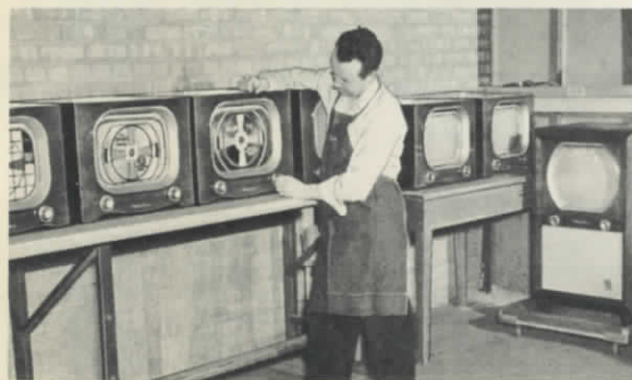
SPOT CHECKING signal reception by service engineers who make daily operating checks of sets which are taken from the assembly line. It's the test that tests all other tests.
