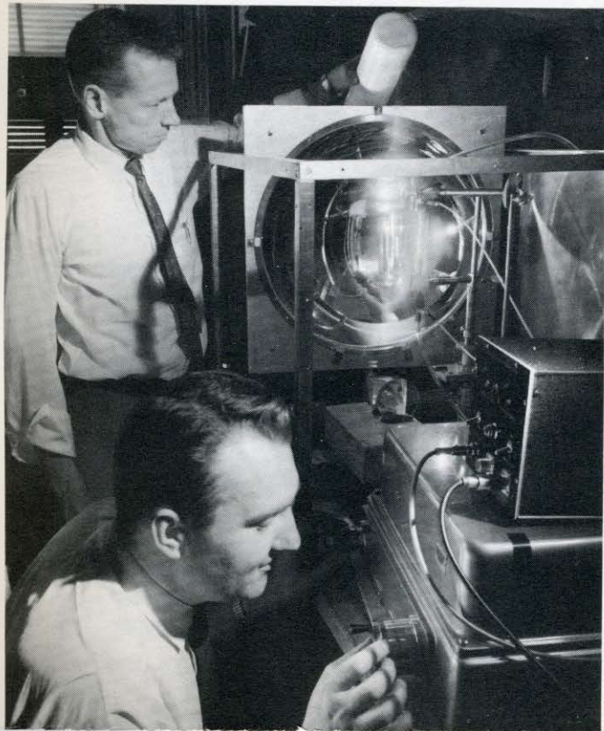
Scientists operate RCA-developed laser requiring less energy than other types to generate infrared beams.
