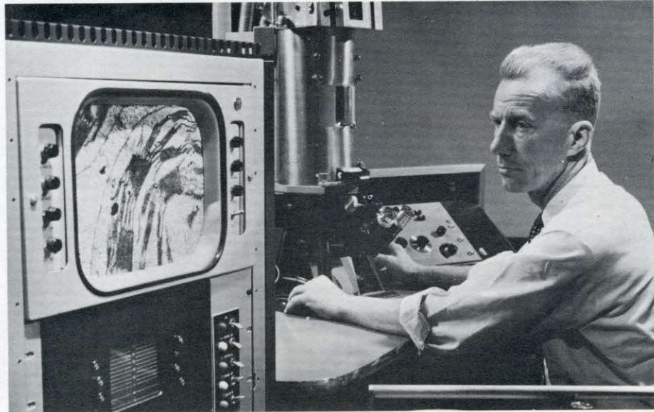
The combination of television with the RCA electron microscope gives scientists more power and flexibility in exploring the molecular structure of matter.
