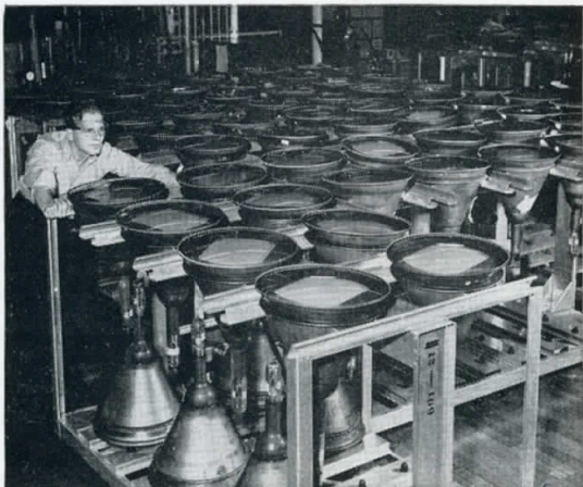
RCA tri-color picture tubes—heart of color television receivers—in pilot production at the RCA plant Lancaster, Pa.
