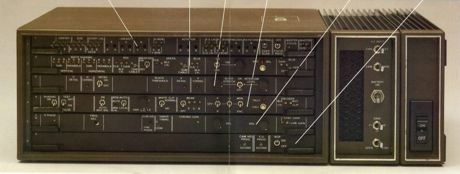
The Remote Control Panel (below) remotes production controls up to 2000 feet from the EU. Controls include paint (red and blue trim), joystick iris and black level, IC volume, IC isolate, black stretch on-off, black stretch control, tally/call, and horizontal and vertical centering. Illuminated indicators include power, operate, sync lock, tally/call, black stretch, and IC isolate.
