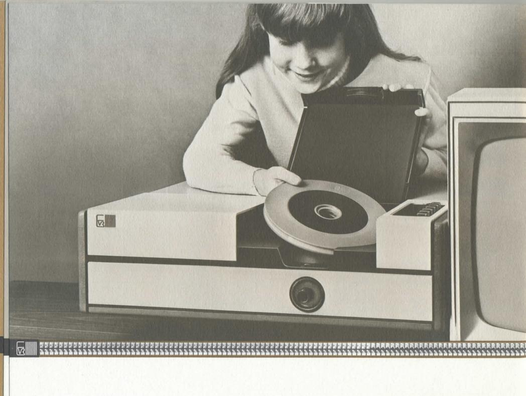
Two basic elements go together to form the EVR™ system—the cartridge and the playback unit.
