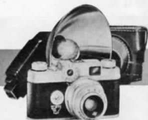
No. C-4—FLASH CAMERA. With a 50 mm f/2.8 coated Argus Cinar anastigmat lens. Takes 36 exposures on a 35 mm cartridge. Lens shutter speed of 1/10 to 1/300 sec. and B. Flash synchronized with 5 and 20 ms. adjustments. Rangefinder and viewfinder combined. Automatic shutter cocking. Clip-on flash unit and bayonet. Convenient Everready case. LIST $99.50.
