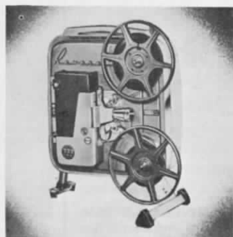
No. P-777 — "CONTEMPORARY" 8mm PROJECTOR. One simple "forward-reverse" control. Built-in safety feature. AC operation. 500 Watt lamp. 3/4" f/1.6 coated lens. LIST $127.50.
